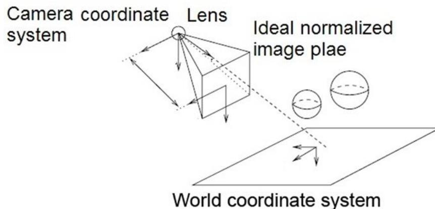
Fig. 1.2 Illustration of the camera model, image in front of the lens to simplify calculations [Courtesy of Maria Magnusson Seger].
