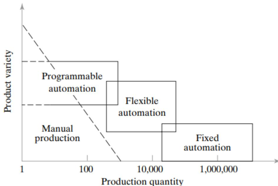
Figure 2.3. Three types of automation relative to production quantity and product variety.
