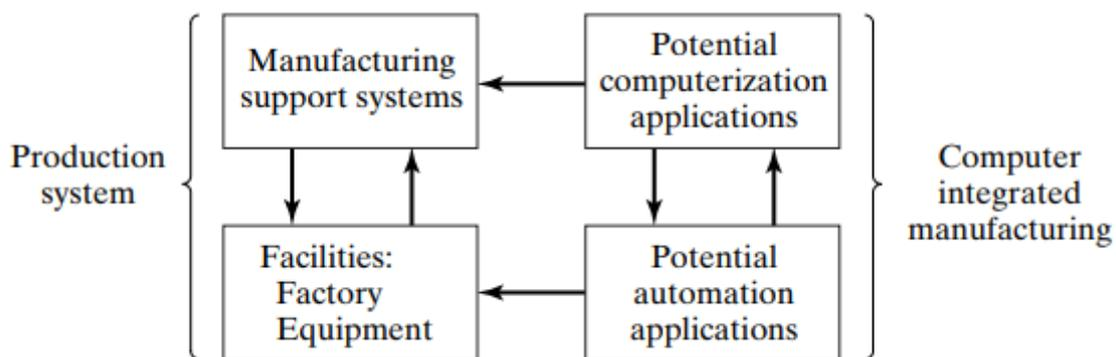
Figure 2.2. Opportunities of automation and computerization in a production system.
