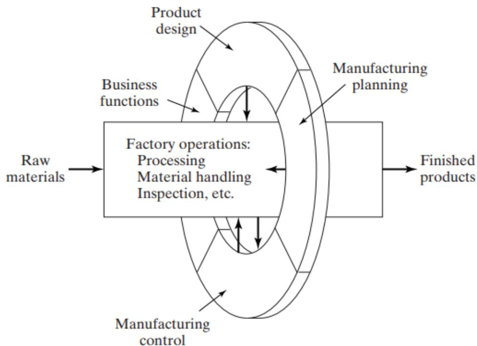
Figure 2.4. Model of manufacturing showing factory operations and the information processing activities for manufacturing support.
