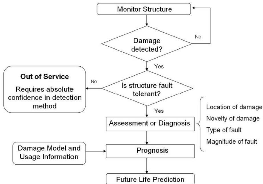
Figure 1: A general flow chart of a SHM system including the 4 stages in which SHM is most commonly divided: Detection, Location, Severity and Prognosis
