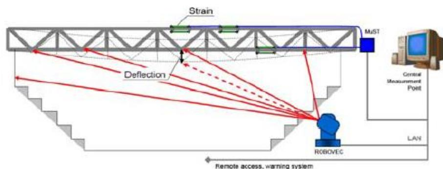
Figure 4: Setup with strain and deflection sensors.
