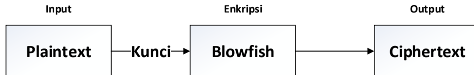
Gambar 6. Diagram Blok Proses Enkripsi File
