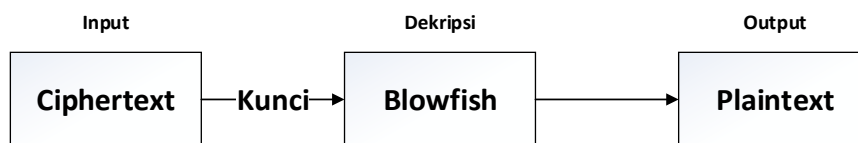
Gambar 8. Diagram Blok Proses Dekripsi File
